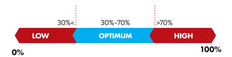
For oprtimum comfort and a healthy indoor environment humidity levels should be maintained between 30% - 70%. Clay plasters naturally help maintain these levels minimising mold and fungal growth within buildings.
